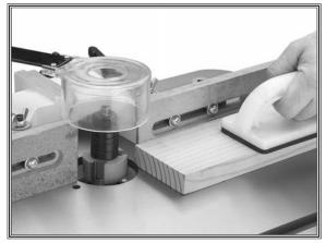
**Figure 16.** Shaper cutter installed on spindle.
