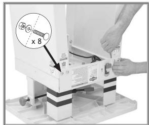
Figure 9. Attaching stand to shaper unit.
