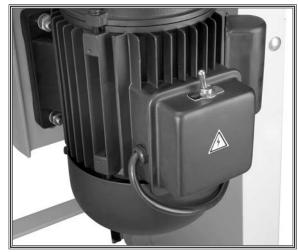
Figure 20. Forward and reverse switch.
