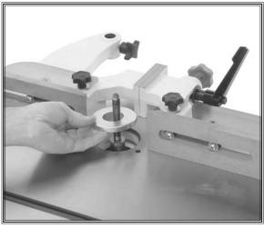
**Figure 23.** Using table insert to keep wood shavings on table.
