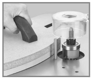
Figure 37. Using starting pin with hold-down jig to support workpiece.
