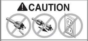
DO NOT modify the provided plug or use an adapter if the plug will not fit the receptacle. Instead, have an electrician install the proper receptacle on a power supply circuit that meets the requirements for this machine.
