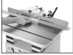
**Figure 22.** Use straightedge to check fence.
